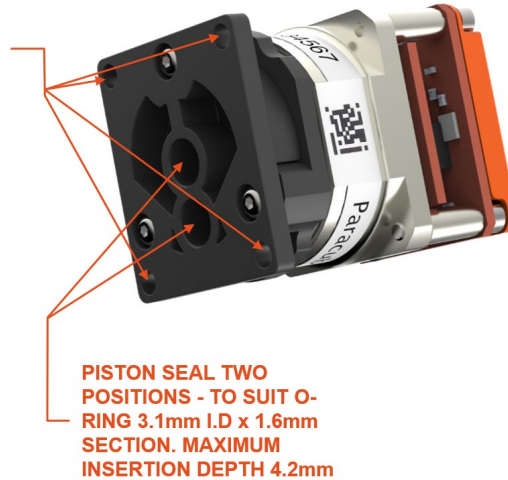
Fig. 4 Flange mounted – gas connection via OEM supplied gas ports
